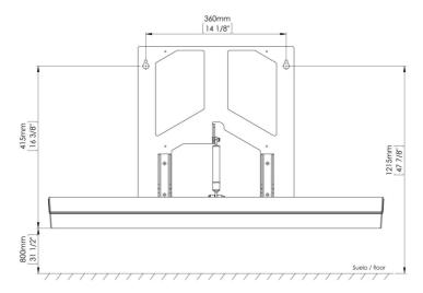
Following the above scheme, using the pencil, mark on the wall the top two holes of the changing station's holding structure. It is very important to make sure that the locations marked with the pencil for the mounting holes are at the same level before drilling the holes.
