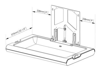
The recommended installation height is 800 mm from the ground to the lowest part of the changing station. The following sketch shows the height at which the holes should be made in order for the changing station to be installed at the recommended height:
