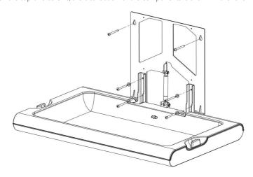
Make sure that the six screws securing the unit to the wall have been properly tightened and that the changing station is firmly fixed to the wall.
