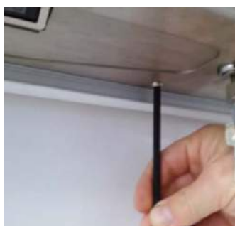
3. Undo the 1st T30V retaining screw
