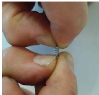
7. Catch 2 coils & stretch spring slightly
