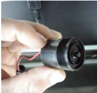
4. Remove diaphragm from solenoid
