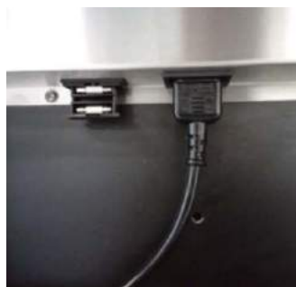
1. Slide open the fuse holder
