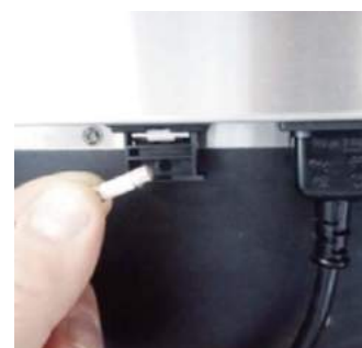
6. Replace the fuse in the holder
