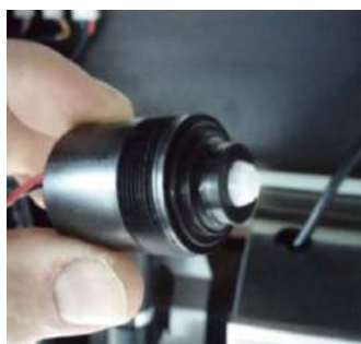
4. Check diaphragm for particles
