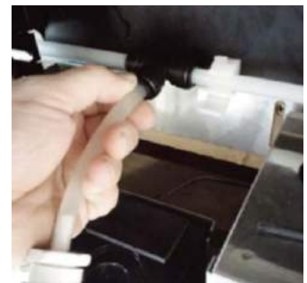
5. Disconnect pump from tee
