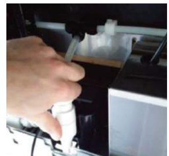
8. Fit new pump into gearbox
