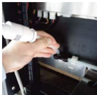
7. Push new pump firmly into tee
