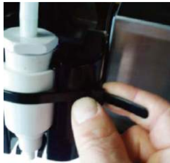
3. Undo cable tie restraining pump
