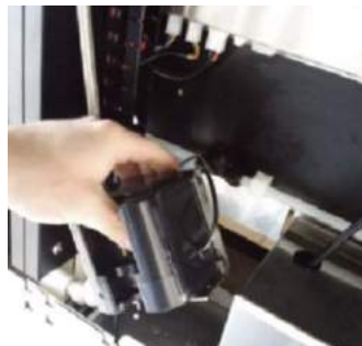
8. Lift out the gearbox
