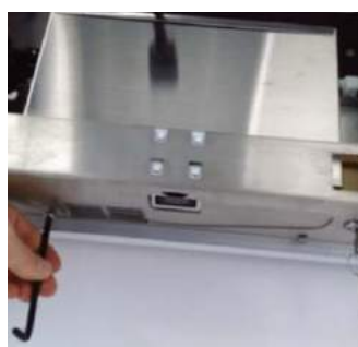
4. Undo the 2nd T30V retaining screw
