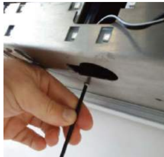
6. Undo the 2 x T20V retaining screws
