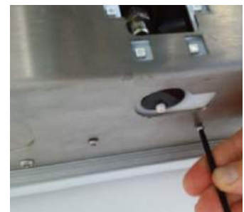
5. Undo the 2 x T20V retaining screws
