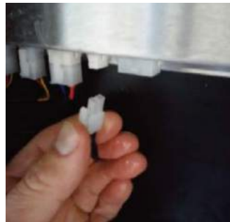
7. Unplug the gearbox from trunking...
