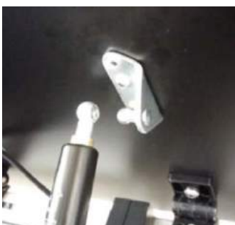
4. Pop top of strut off the bracket
