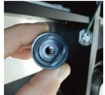
5. Remove pin and check spring
