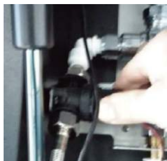
3. Unscrew the solenoid from body
