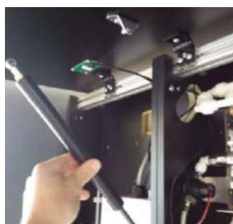
Support the strut and lower it
