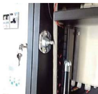
5. Pop bottom of strut off the bracket
