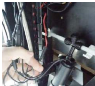
7. Remove all the dispenser wiring
