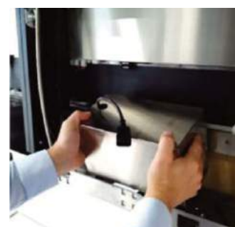
5. Lift out the dryer unit
