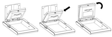
Open the liner dispenser with the special key provided. The four holes for mounting the liner dispenser on the holding structure of the changing station will be visible.
