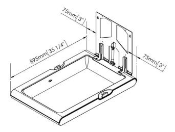
The recommended installation height is 800 mm from the ground to the lowest part of the changing station. The following sketch shows the height at which the holes should be made in order for the changing station to be installed at the recommended height:
