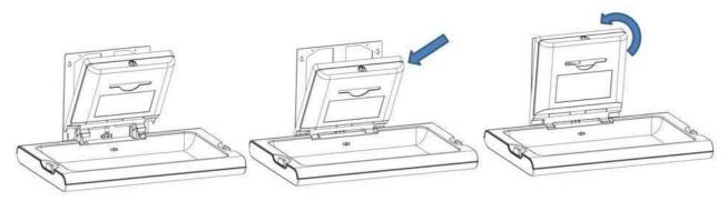
Open the liner dispenser with the special key provided. The four holes for mounting the liner dispenser on the holding structure of the changing station will be visible.
