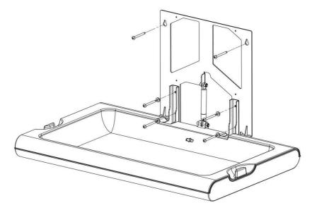
Make sure that the six screws securing the unit to the wall have been properly tightened and that the changing station is firmly fixed to the wall.
