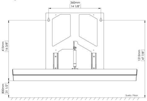
Following the above scheme, using the pencil, mark on the wall the top two holes of the changing station's holding structure. It is very important to make sure that the locations marked with the pencil for the mounting holes are at the same level before drilling the holes.
