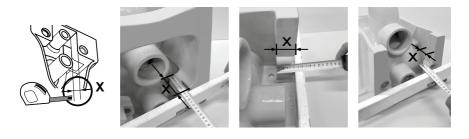
Measure the thickness of the ceramic 'X' from the support point of the WB9 B on the ceramic to the outermost point of the sanitary ware which will rest on the wall.
